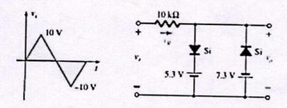
ii. Determine the currents  $I_1, I_2, I_3, \, I_4$  and  $V_o$  for the network shown:
